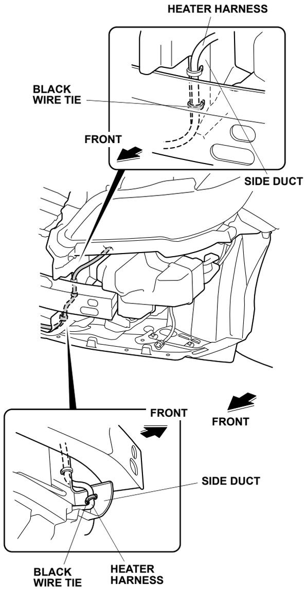
26. Secure the heater harness to the vehicle harness with one wire tie.
