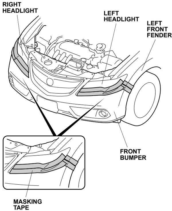
6. Repeat step 5 to apply masking tape to the right side of the vehicle.
