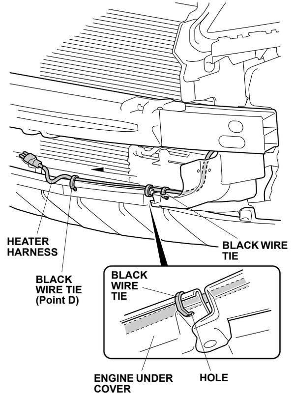
24. Secure the heater harness to the side duct and engine under cover with two black wire ties.
