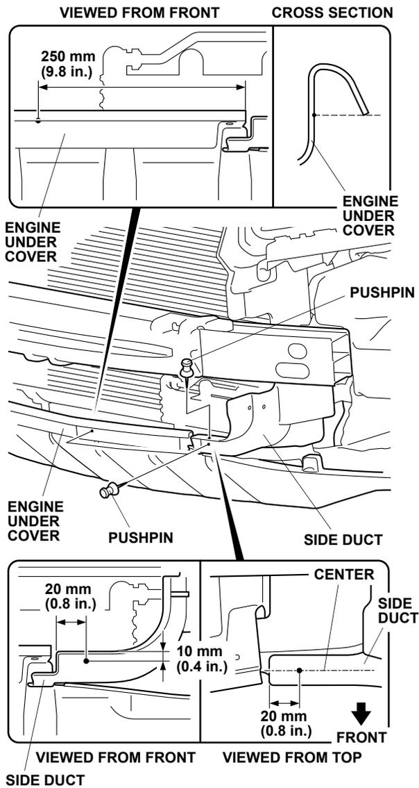
13. While wearing eye protection, drill the three pierced marks on the side duct and engine under cover with a 3 mm drill bit, then enlarge the three holes with a 7 mm drill bit. Remove any burrs. Wrap tape around each drill bit 7 mm away from the tip or use a drill stop.
