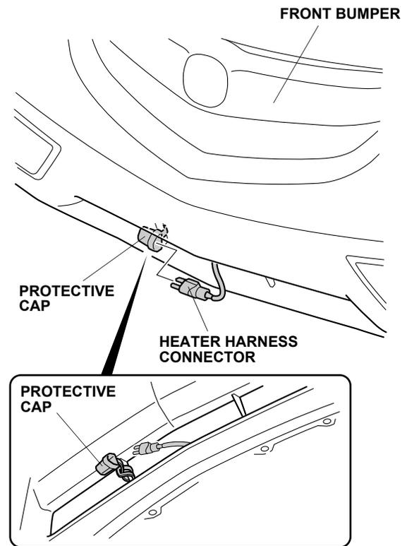
31. Install the heater harness connector into the protective cap.
