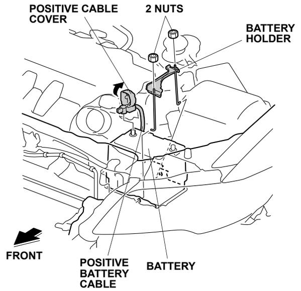
10. Remove the battery holder (two nuts).
