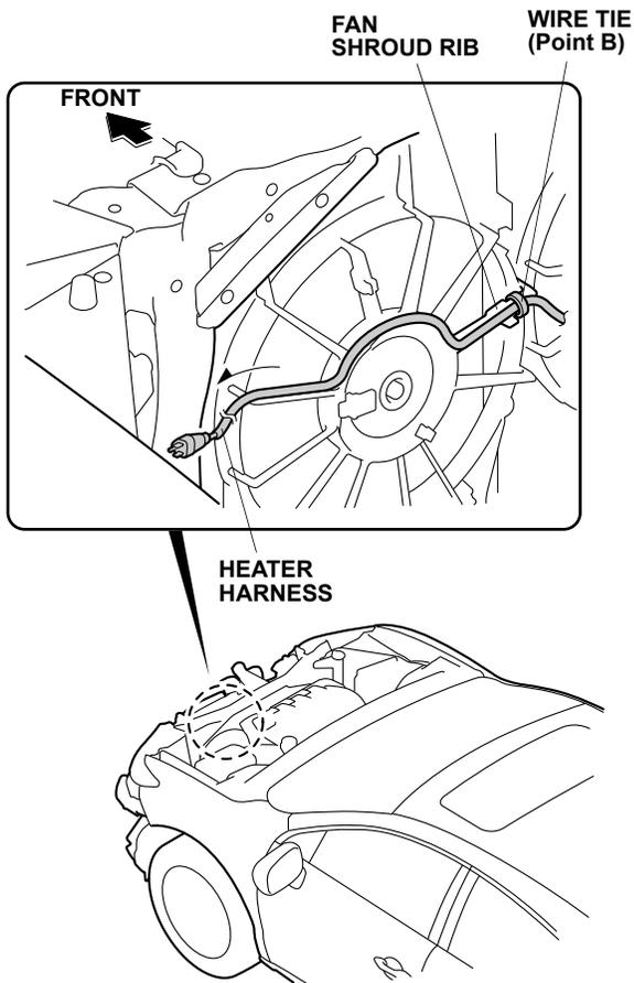
21. Continue routing the heater harness along the vehicle harness.
