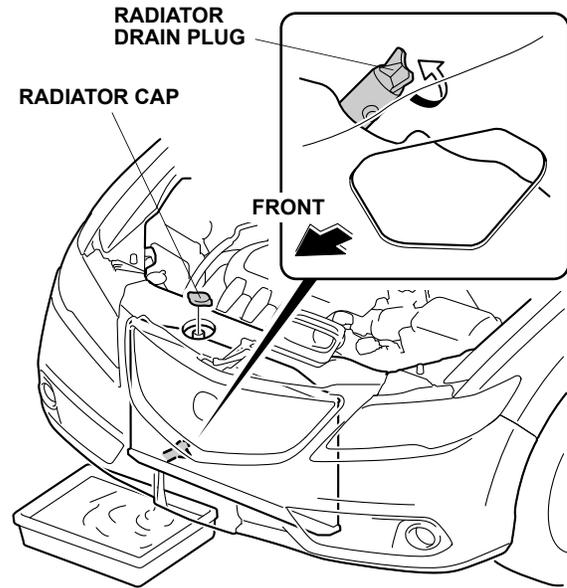
4. After the coolant drains, reinstall the radiator cap to prevent dirt and contamination from entering the radiator.
